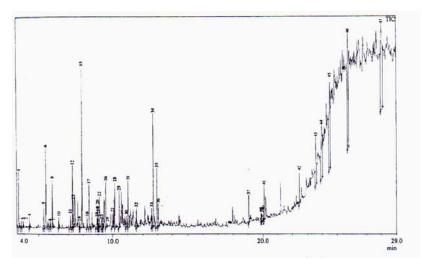
Figure 1. Gas Chromatogram of Used Engine Oil Before Biodegradation.
