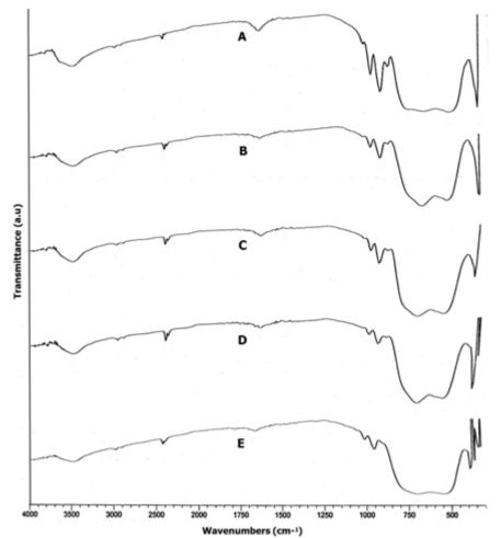
**Fig 2.** FTIR spectrum of  $H_4[\alpha$ -SiW<sub>12</sub>O<sub>40</sub>]/TiO<sub>2</sub> under various weight of TiO<sub>2</sub> (A: 0.25g; B: 0.50 g; C: 0.75 g; D: 1.00 g; and E: 1.25 g)
