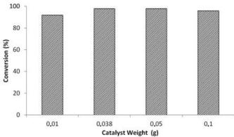
Fig 6. Effect of catalyst weight in the oxidation of cyclohexane using  $H_4[\alpha$ -SiW<sub>12</sub>O<sub>40</sub>]/TiO<sub>2</sub>
