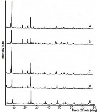
**Fig 3.** XRD powder pattern of  $H_4[\alpha$ -SiW<sub>12</sub>O<sub>40</sub>]/TiO<sub>2</sub> under various weight of TiO<sub>2</sub> (A: 0.25 g; B: 0.50 g; C: 0.75 g; D: 1.00 g; and E: 1.25 g)
