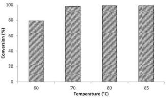
Fig 5. Effect of temperature in the oxidation of cyclohexane using  $H_4[\alpha$ -SiW<sub>12</sub>O<sub>40</sub>]/TiO<sub>2</sub>
