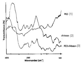
**Fig 1.** FT-IR spectrum of [1] PEO [2] Chitosan and [3] PEO-chitosan hydrogel
