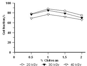
**Fig 2.** Effect of chitosan concentration on the gel fraction of PEO-chitosan hydrogels at different radiation doses with 5% PEO
