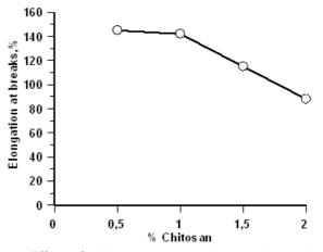
**Fig 4.** Effect of chitosan concentration on elongation at break of PEO-chitosan hydrogels (formed at 20 kGy)
