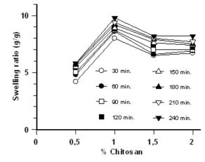
**Fig 3.** Effect chitosan concentration on the swelling ratio of PEO-chitosan hydrogels (formed at 20 kGy) in different time
