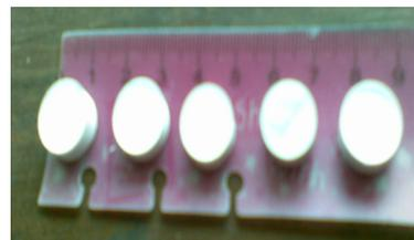
Fig 1. The pellets of borosilicate sintered at 900 °C
