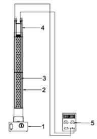
Fig 1. Electrocatalytic tube reactor consists of (1) magnetic stirrer, (2) PVC tube, (3) Ti/RulrO<sub>2</sub> cylindrical anode, (4) Fe cathode and (5) DC power supply
