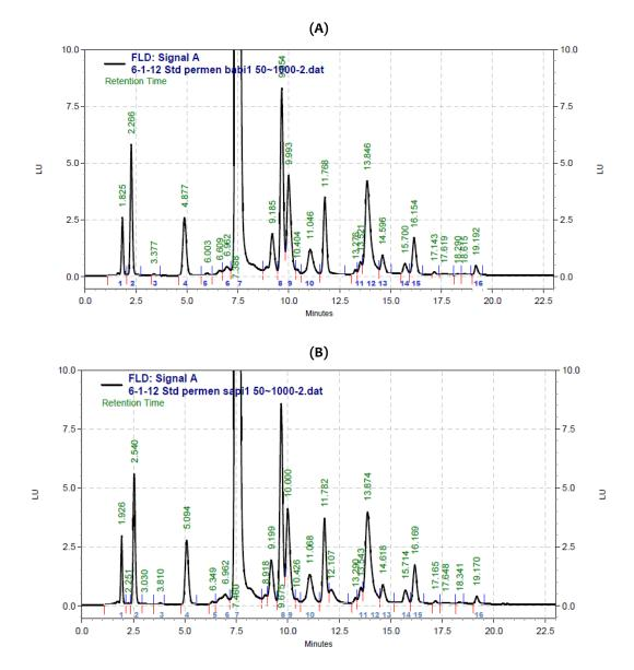
Figure 2. Chromatogram of amino acids in laboratory prepared soft candy made from porcine (A) and bovine (B) gelatins from Sigma after hydrolysis and pre-column derivatization. 1: aspartic acid, 2: glutamic acid; 3: asparagine; 4: serine and cysteine; 5: glutamine; 6: histidine; 7: glycine and threonine, 8: arginine; 9: alanine; 10: tyrosine; 11: methionine and tryptophan; 12: valine; 13: phenylalanine; 14: isoleucine; 15: leucine; 16: lysine.
