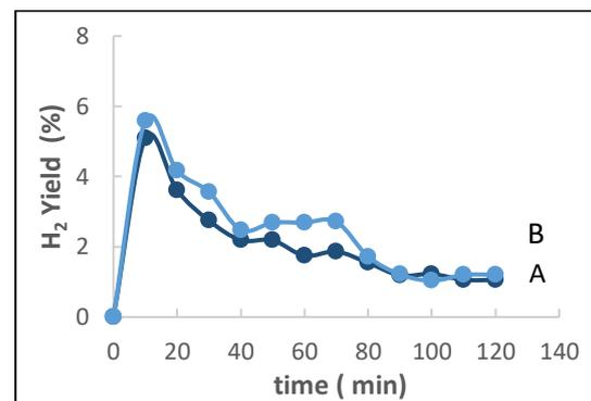
**Fig. 5:** H<sub>2</sub> yield of: (A) Ni/CaO- $\gamma$ -Al<sub>2</sub>O<sub>3</sub> (B) Ni/CaO- $\gamma$ -Al<sub>2</sub>O<sub>3</sub>@Ru core shell
