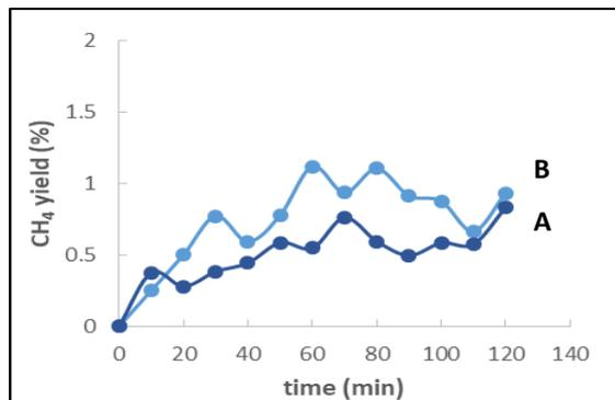
**Fig. 6:** CH<sub>4</sub> yield of: (A) Ni/CaO- $\gamma$ -Al<sub>2</sub>O<sub>3</sub> (B) Ni/CaO- $\gamma$ -Al<sub>2</sub>O<sub>3</sub>@Ru core shell
