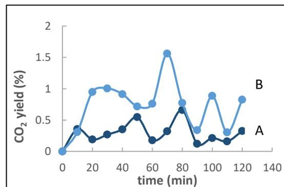
**Fig. 8:** CO<sub>2</sub> yield of: (A) Ni/CaO- $\gamma$ -Al<sub>2</sub>O<sub>3</sub> (B) Ni/CaO- $\gamma$ -Al<sub>2</sub>O<sub>3</sub>@Ru core shell
