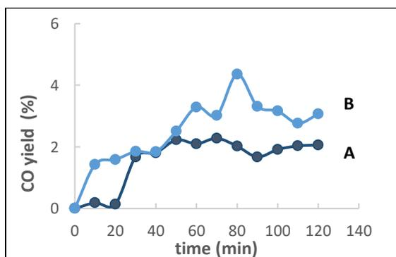
**Fig. 7:** CO yield of: (A) Ni/CaO- $\gamma$ -Al<sub>2</sub>O<sub>3</sub> (B) Ni/CaO- $\gamma$ -Al<sub>2</sub>O<sub>3</sub>@Ru core shell
