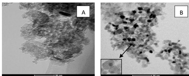
**Fig. 2:** TEM morphology of (A) Ni/CaO- $\gamma$ -Al<sub>2</sub>O<sub>3</sub>, (B) Ni/CaO- $\gamma$ -Al<sub>2</sub>O<sub>3</sub>@Ru core-shell in 50 nm scale
