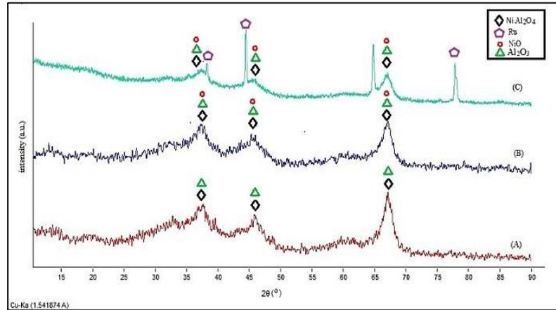
**Fig. 1:** (A) XRD patterns of CaO- $\gamma$ -Al<sub>2</sub>O<sub>3</sub>; (B) Ni/CaO- $\gamma$ -Al<sub>2</sub>O<sub>3</sub>; (C) Ni/CaO- $\gamma$ -Al<sub>2</sub>O<sub>3</sub>@Ru
