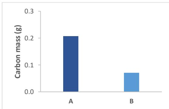
**Fig. 4:** Carbon deposit in: (A) Ni/CaO- $\gamma$ -Al<sub>2</sub>O<sub>3</sub> (B) Ni/CaO- $\gamma$ -Al<sub>2</sub>O<sub>3</sub>@Ru core shell
