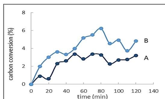
**Fig. 3:** Carbon conversion of steam reforming by using: (A) Ni/CaO- $\gamma$ -Al<sub>2</sub>O<sub>3</sub> (B) Ni/CaO- $\gamma$ -Al<sub>2</sub>O<sub>3</sub>@Ru core shell
