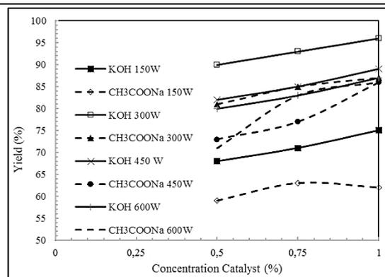
**Fig. 3.** Effect of catalyst concentration on yield of biodiesel
