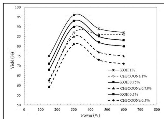
**Fig. 2.** Effect of microwave power on biodiesel yield
