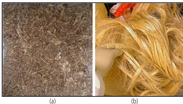
Figure 1. Chopped bagasse (a) and abaca bundles (b) were alkali-treated and pressed into fiber sheets, which will be laminated later to fabricate hybrid NFRP samples.
