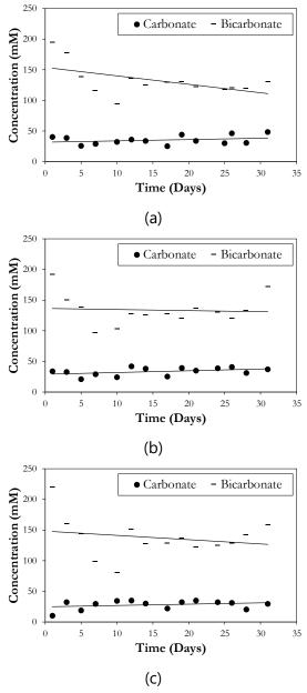
**Fig. 7** Concentration profile of carbonate and bicarbonate in BICCAPS with Na<sub>2</sub>CO<sub>3</sub> under (a) Modified Zarrouk's, (b) NPK-based, and (c) NPK-A<sub>5</sub> media
