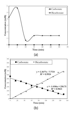
**Fig. 2** Gas Absorption Response of (a) Control System, (b) Sodium Carbonate Solution
