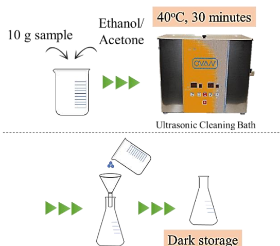
Fig. 2: Steps of sonication extraction diagram
