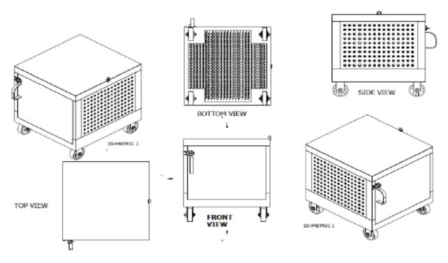
Figure 3. Showed autographic views of the designed tomato charcoal cooler storage bin
