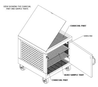
Figure 1. Developed tomato charcoal cooler bin
