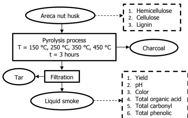
Figure 2. Flowchart of the production stage of liquid smoke *Areca* nut husk
