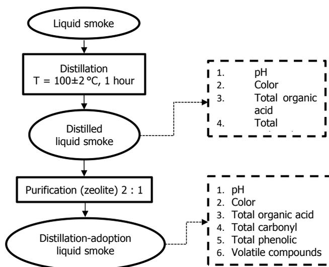
Figure 3. Flowchart of liquid smoke purification process
