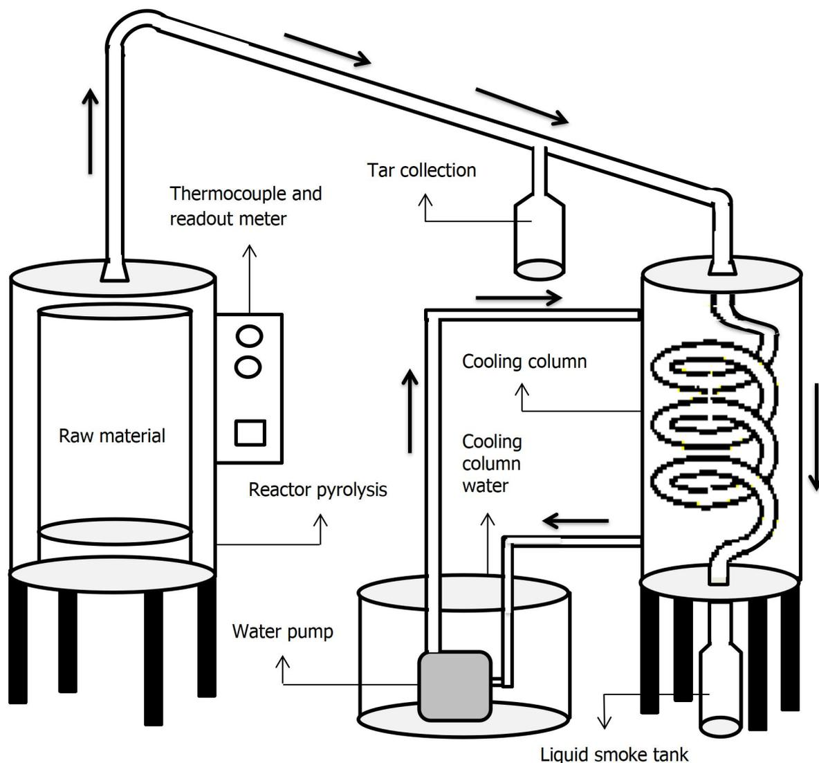
Figure 1. Schematic diagram of experimental apparatus
