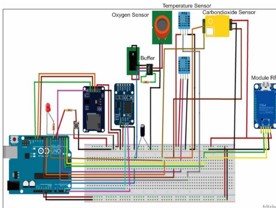
Figure 2. Respiratory chamber wiring diagram
