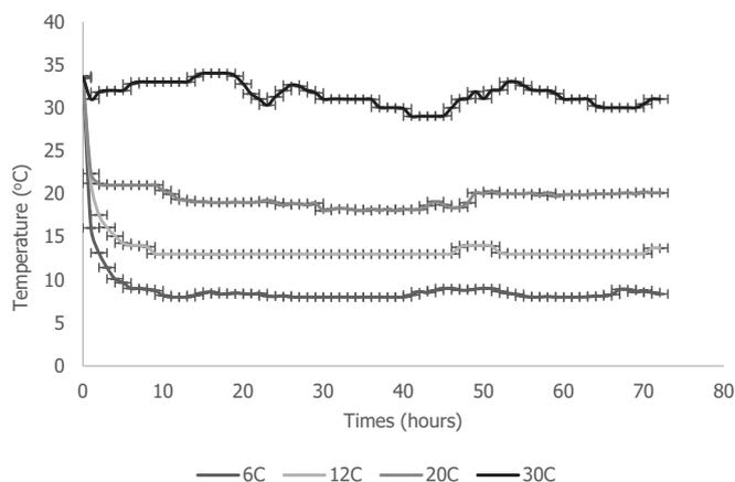
Figure 3. Temperature behavior in the respiratory chamber at various set-up points
