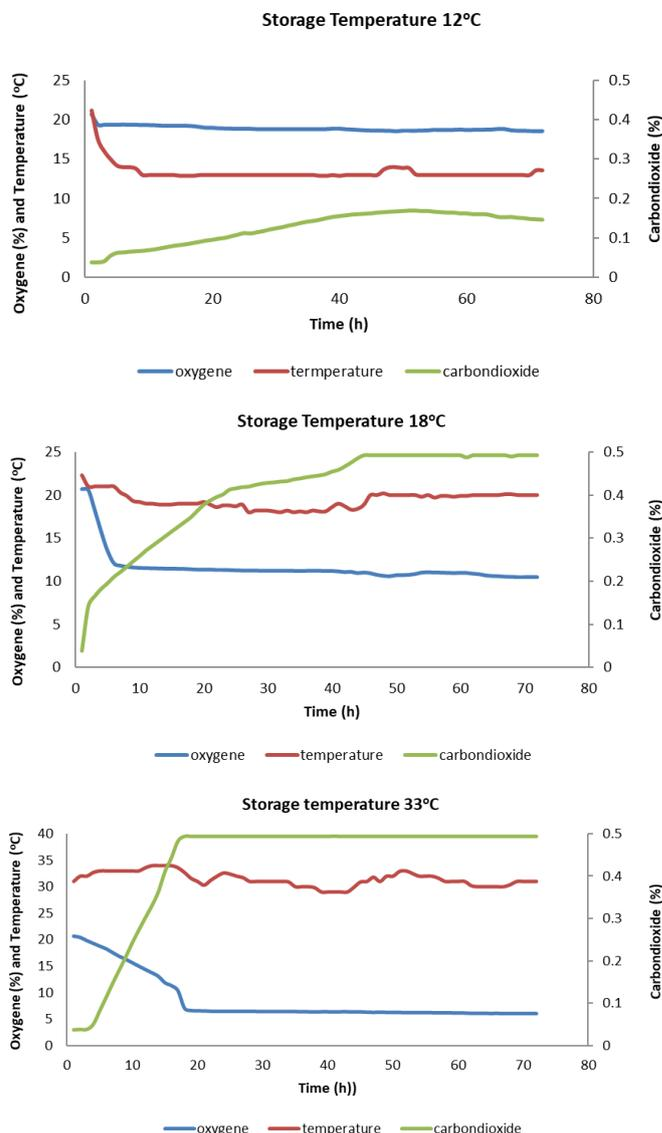
Figure 5. Respiration data acquisition measurement at storage temperature: a) 12 °C, b) 18 °C, and c) 33 °C
