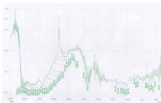
Figure 4. Infra red (IR) spectrum at tapioca starch of crosslinked acylation STPP 5% and stearic acid 2% of substituted Nagara bean flour with 50:50 ratio
