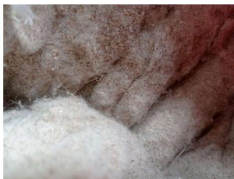
Figure 2. Fan Open End Cotton Waste
