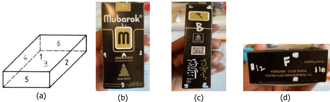
Figure 2. Illustration and Implementation View of Packaging Areas Classification Based on ISO 2206:1987 (a) Illustration of Packaging (b) Top View (c) Right Side View (d) Front View
