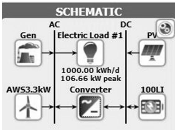
Figure 7. HOMER Simulation Schematic
