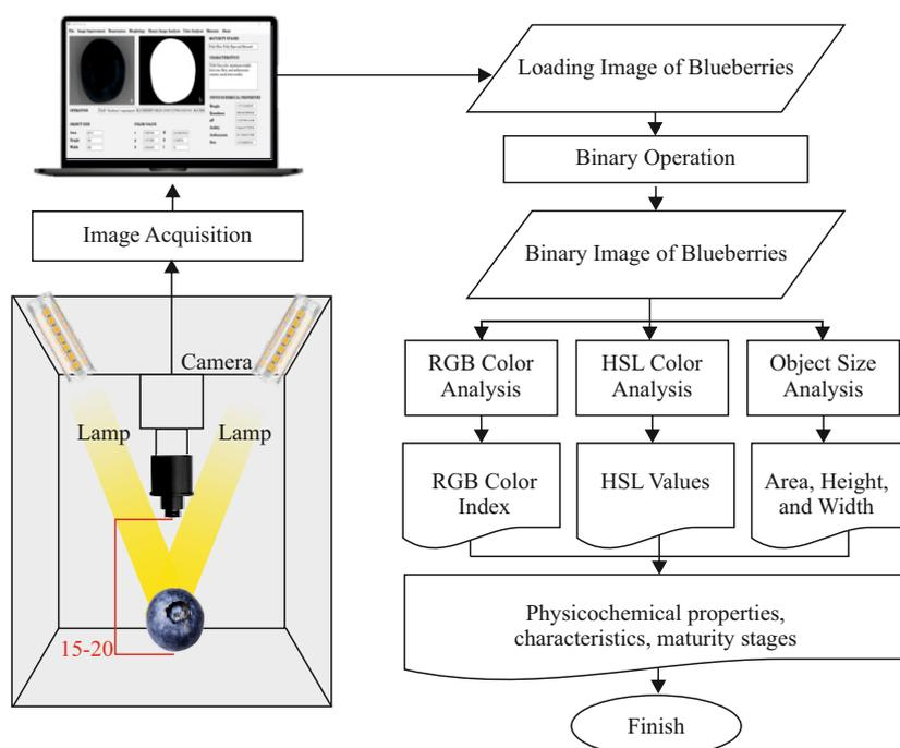
Figure 1. Image processing diagram along with the data stream and camera configuration.
