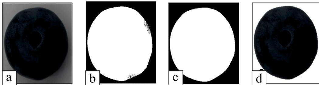
Figure 2. Image processing applied to extract chromatic and geometric of blueberries; (a) original image captured, (b) binary image obtained by grayscale thresholding process, (c) binary image after opening and closing, and (d) result of masking for background elimination before color extraction.
