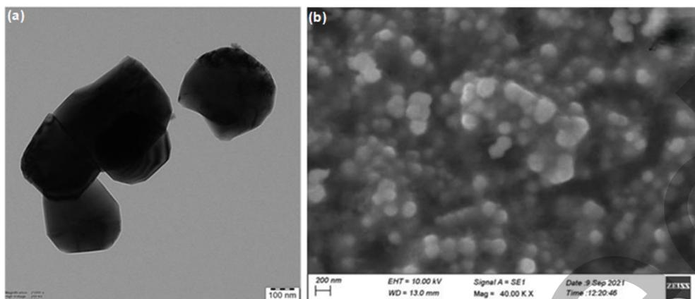
Fig 4. Micrograph of (a) HRTEM and (b) SEM of nanochitosan (retrieved from Duraisamy et al. [58])
