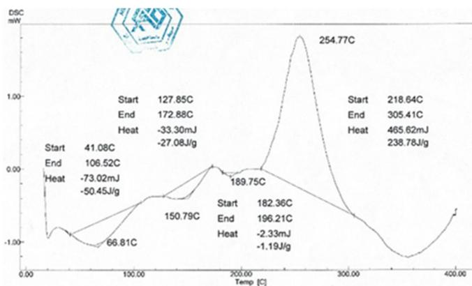
Fig S15. DSC curve of Ni-complex
