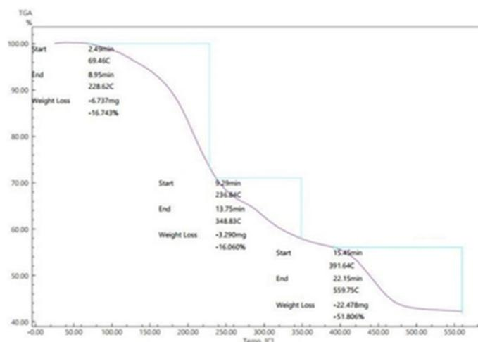
Fig S12. TGA curve of Ni-complex
