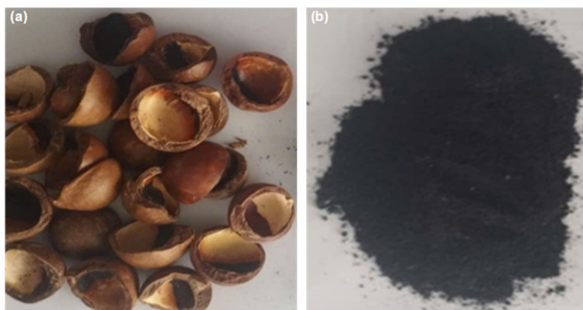
Fig 1. (a) Raw materials and (b) biochar from macadamia husk
