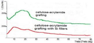
Fig 3. X-ray diffractograms of grafted cellulose and grafted cellulose with silica added
