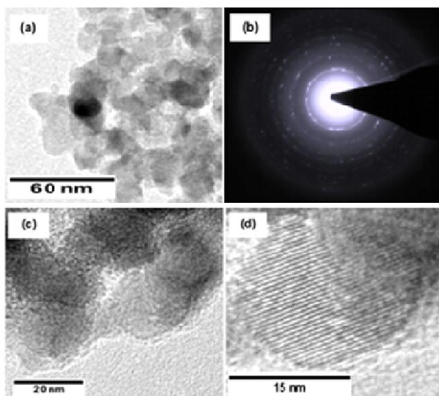
**Fig 3.** Typical morphology images of TiO<sub>2</sub>: (a) bright-field-TEM, (b) Selected area electron diffraction (SAED), (c) high resolution TEM, and (d) enlarged lattice fringes
