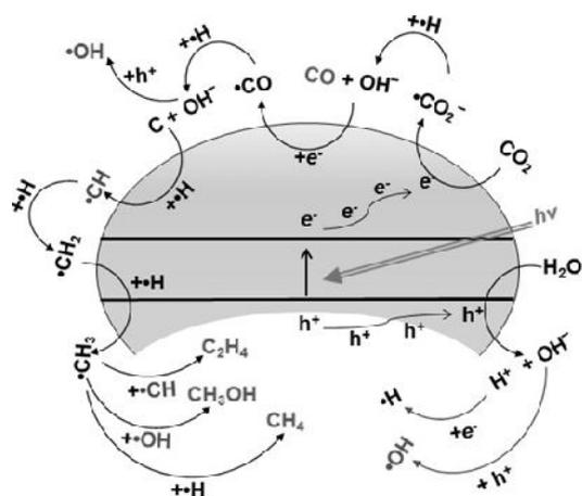
**Fig 5.** A reaction pathway for the product formation on TiO<sub>2</sub> surface during the photocatalytic CO<sub>2</sub> reduction
