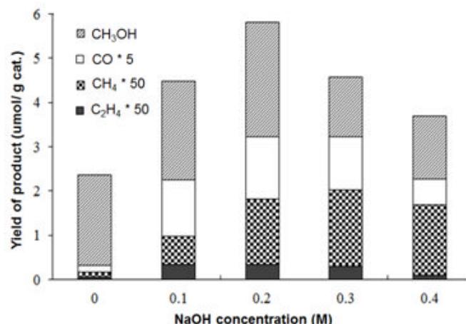
**Fig 6.** The influence of NaOH concentration on the yield of photocatalytic products
