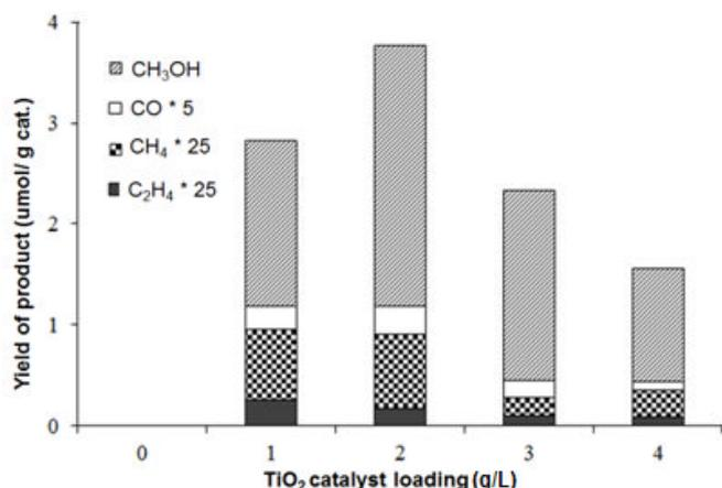
**Fig 7.** The influence of photocatalyst dosage on the yield of photocatalytic products
