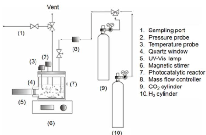
**Fig 1.** Schematic of experimental setup for CO<sub>2</sub> photocatalytic reduction
