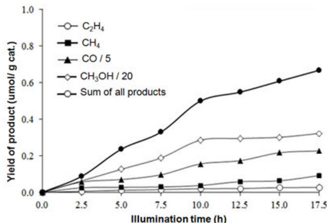
**Fig 11.** Illumination time dependence of the yield of photocatalytic products
