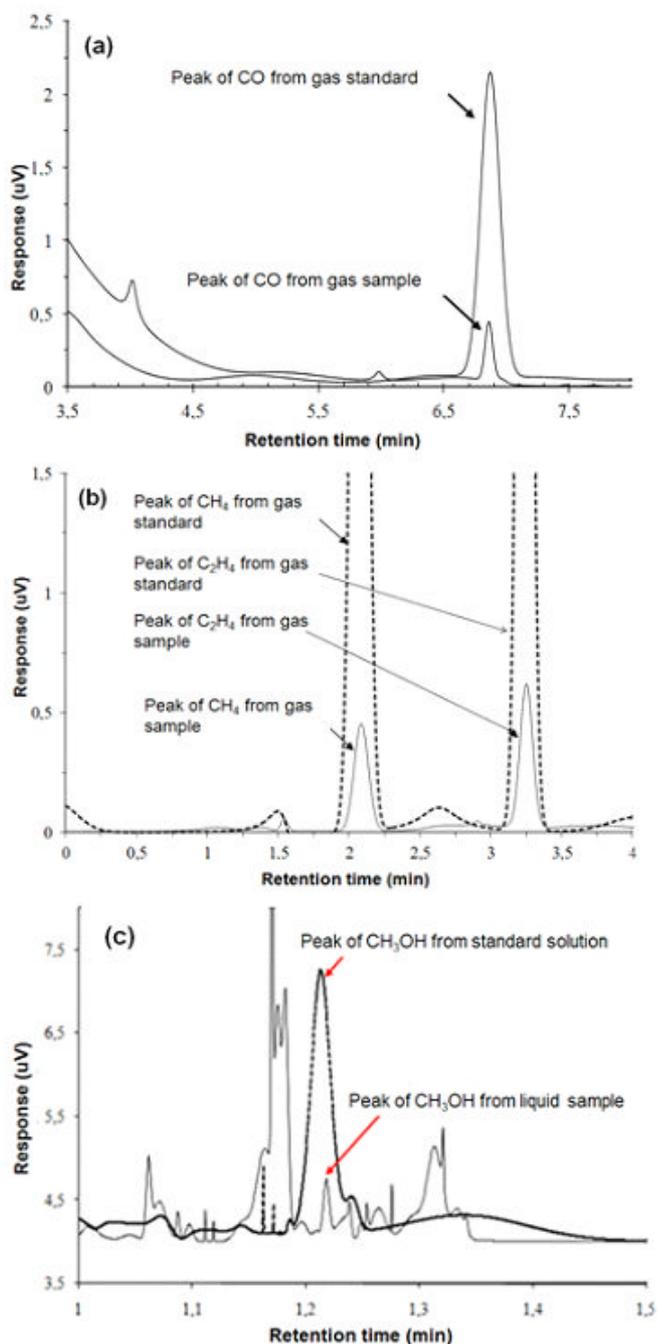
**Fig 4.** The typical chromatogram of the standard and detected products: (a) CO, (b) CH<sub>4</sub> and C<sub>2</sub>H<sub>4</sub>, and (c) CH<sub>3</sub>OH
