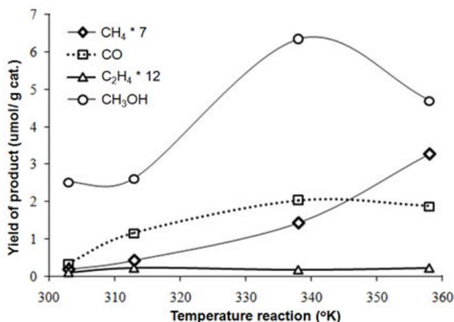
**Fig 10.** The influence of temperature on the yield of photocatalytic products
