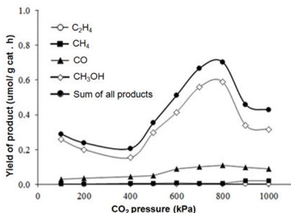
**Fig 9.** The influence of CO<sub>2</sub> pressure on the yield of photocatalytic products
