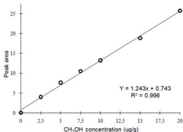
**Fig 2.** The calibration curve for CH<sub>3</sub>OH in standard solutions with excellent linearity measured using GC-FID
