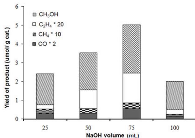
**Fig 8.** The influence of volume of the reaction media on the yield of photocatalytic products
