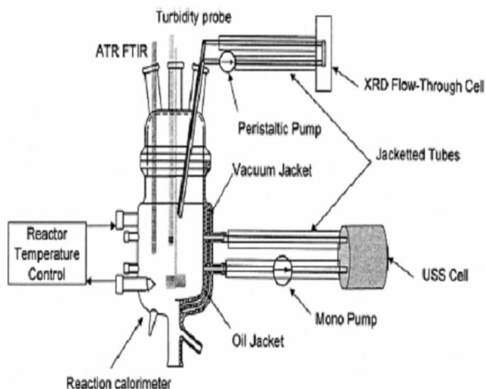
**Fig 1.** Schematic of the 2-litre batch crystallizer integrating the in-situ process analytical techniques of turbidity and ATR FTIR immersion probes, ultrasonic spectroscopy, and X-ray diffraction flow-through cells.
