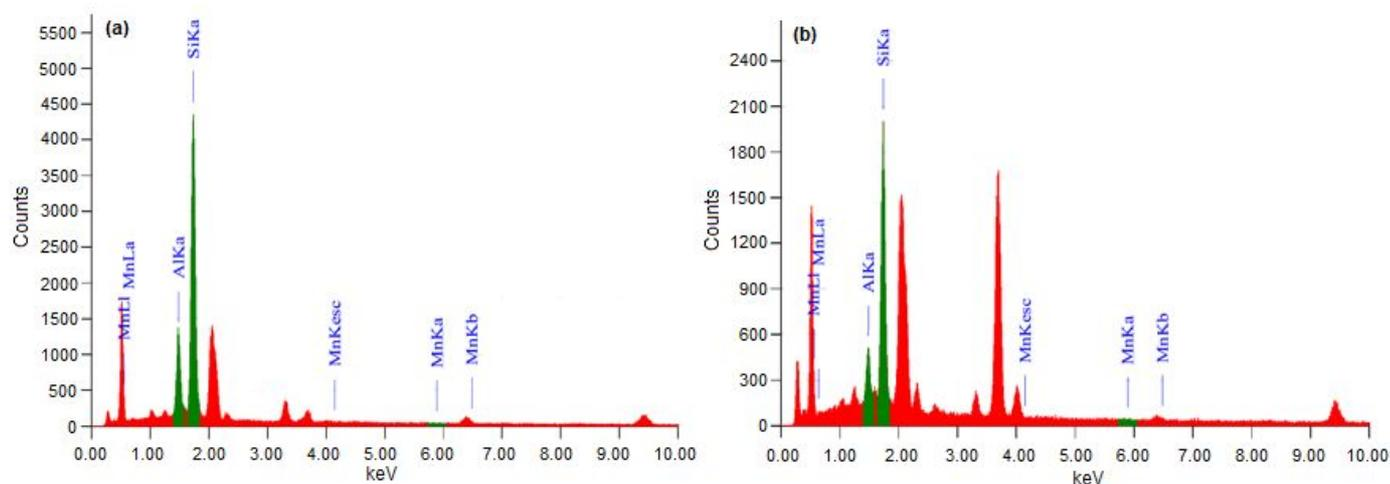
**Fig 5.** EDX spectra of SRB biofilm attached on zeolite particle after interacting with manganese in the continuous reactor after 5 days operation (a) and 9 days operation (b)
