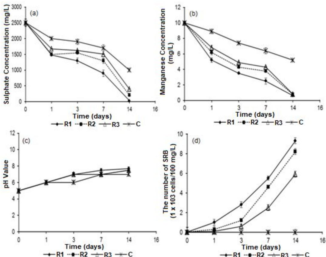
**Fig 1.** Variation sulphate concentrations (a), manganese concentrations (b), pH values (c) and the number of SRB cells (d) during batch experiments of bioreactor using synthetic wastewater which treated by zeolite R1: diameter size 0.4-0.6 cm, R2: 0.6-0.8 cm, R3: 0.8-1.2 cm and C: without treatment
