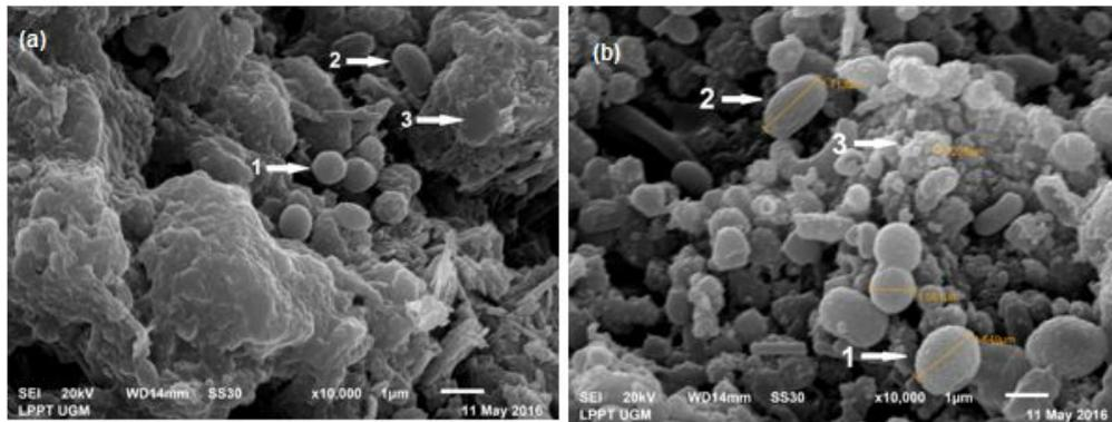
**Fig 4.** Developed biofilm of SRB on the zeolite surface in the continuous reactor after a 5 days (a) and 9 days (b) operation, 1: coccoid form bacterium cell; 2: bacillary form bacterium cell; 3: exopolysaccharide (EPS). Photographs were taken at 10,000× amplification
