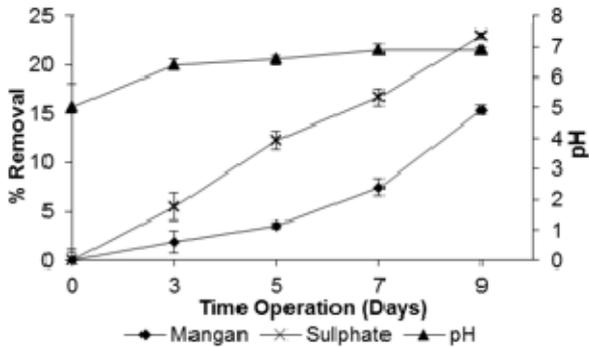
**Fig 2.** Removal of sulphate, manganese concentrations and pH values of effluent during anaerobic continuous bioreactor operation
