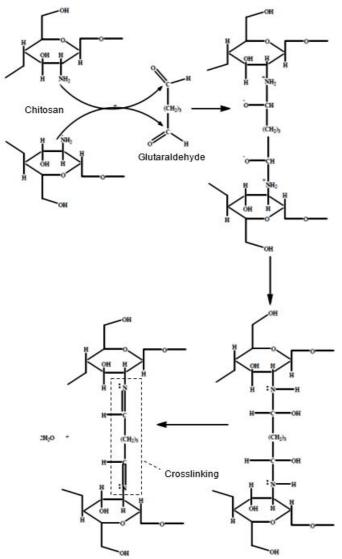
**Fig 2.** Crosslink of chitosan and glutaraldehyde, and interaction with PVFD
