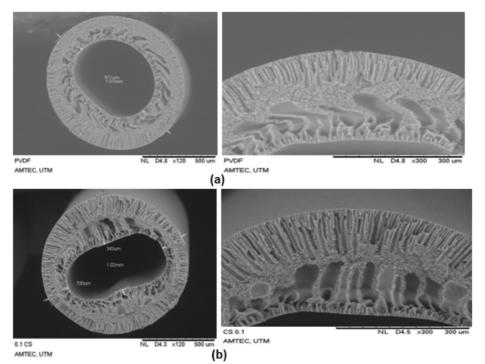
Fig 4. SEM images of cross section of (a) uncoated and (b) coated hollow fiber membrane
