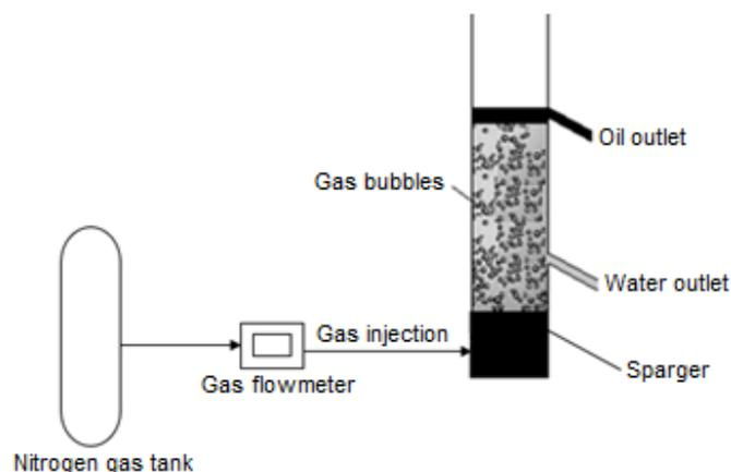
Fig 1. Schematic diagram of the flotation process
