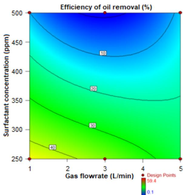
**Fig 5.** Contour plots for the effect of surfactant and gas flow rate at a high polymer concentration (900 ppm) at 10 min flotation duration
