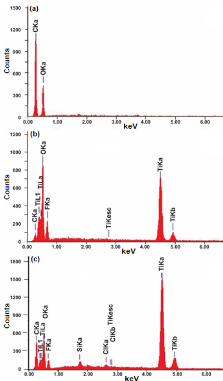
**Fig 7.** EDS spectrum of (a) the pure bamboo timber, (b) TiO<sub>2</sub>-coated bamboo timber, and (C) superhydrophobic bamboo timber
