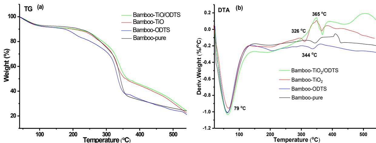
**Fig 8.** TG-DTA curves of superhydrophobic bamboo timber,  $\text{TiO}_2$ -coated bamboo timber, ODTS-coated bamboo timber, and pure bamboo timber
