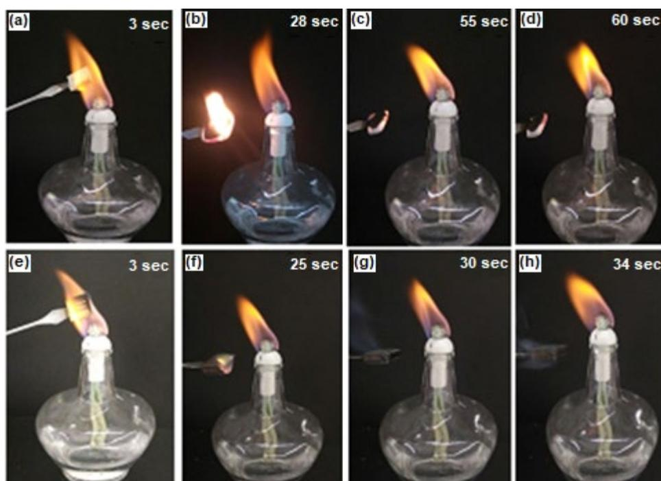
Fig 11. Flammability test of (a-d) pure bamboo timber, and (e-h) superhydrophobic bamboo timber
