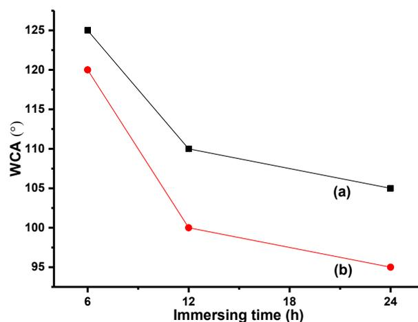
Fig 10. The water contact angle curve of superhydrophobic bamboo timber after immersing in (a) acid and (b) base solution
