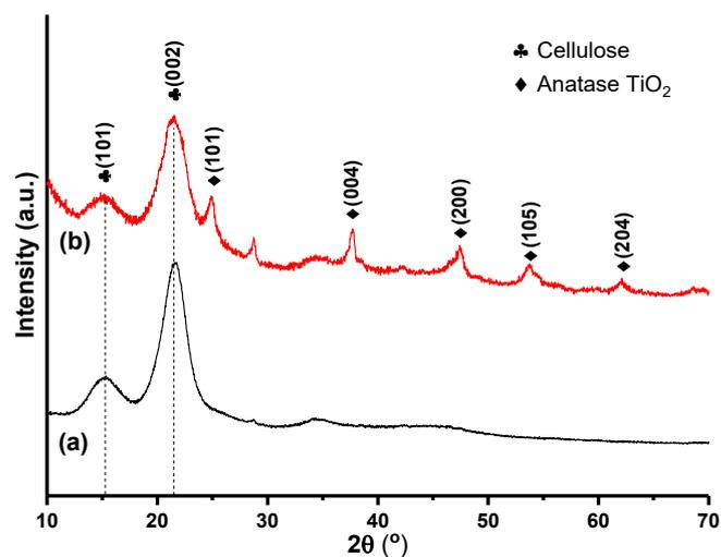
**Fig 4.** XRD Patterns of (a) the pure bamboo timber, (b) the  $\text{TiO}_2$ -coated bamboo timber
