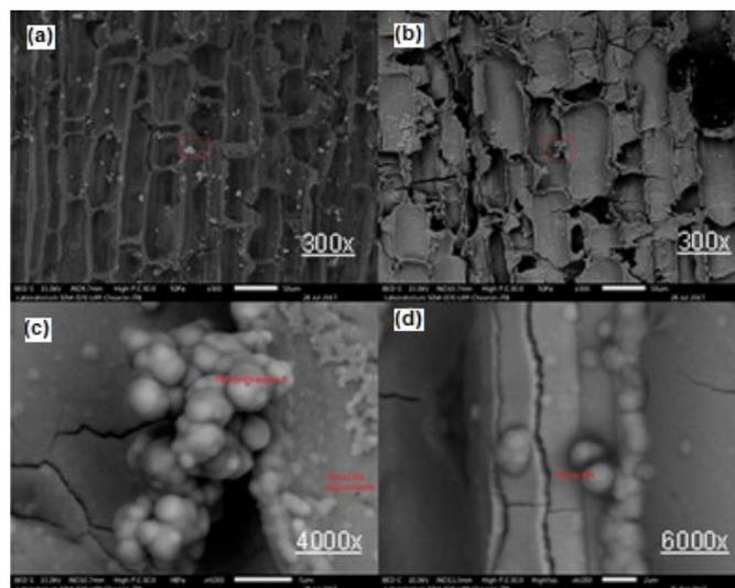
Fig 6. Images SEM of (a) pure bamboo timber (b)  $\text{TiO}_2$ -coated bamboo timber (c) high magnification for images b (d) superhydrophobic bamboo timber
