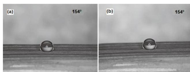
**Fig 9.** The water contact angle of superhydrophobic bamboo timber (a) before and (b) after the scratch test
