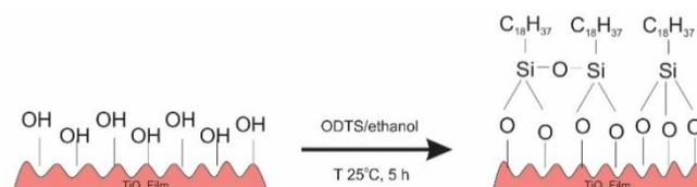
Fig 2. The reaction of superhydrophobic surface fabrication
