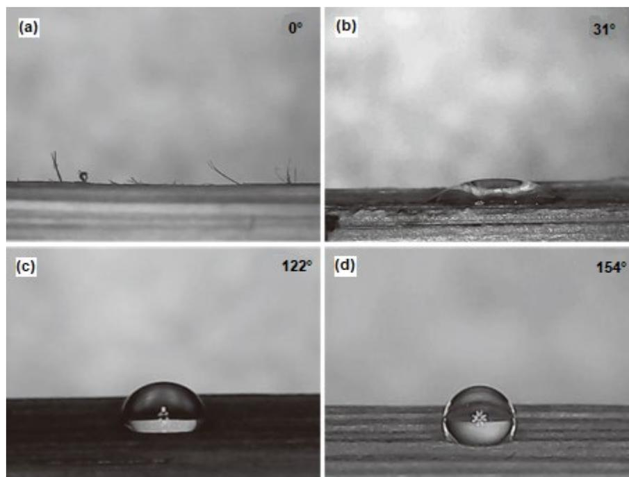
**Fig 3.** Digital images of the water droplets on the surface of (a) pure bamboo timber, (b)  $\text{TiO}_2$ -coated bamboo timber, (c) ODTS-coated bamboo timber, and (d) superhydrophobic bamboo timber
