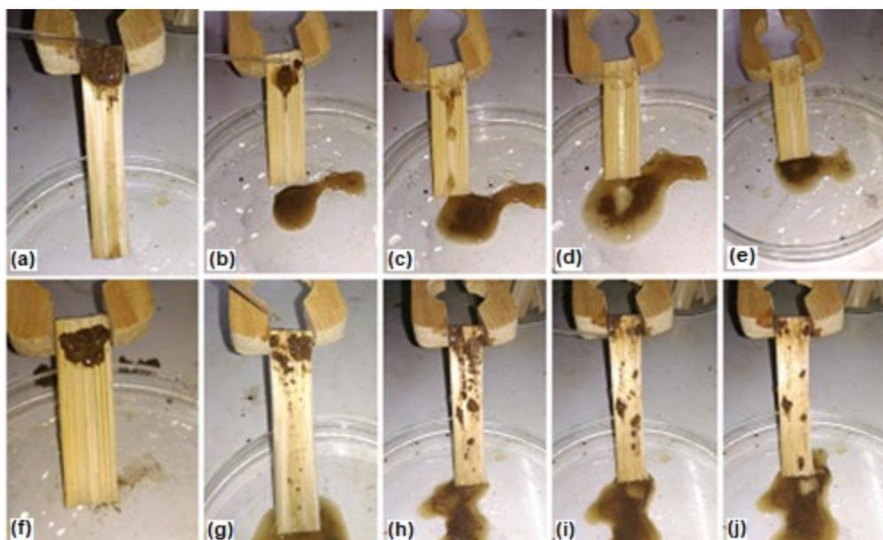
Fig 12. The self-cleaning property test of (a-e) superhydrophobic bamboo timber, and (f-j) pure bamboo timber
