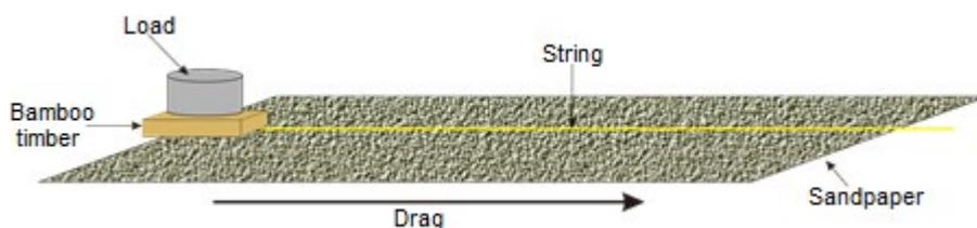
Fig 1. Scheme of the scratch test procedures
