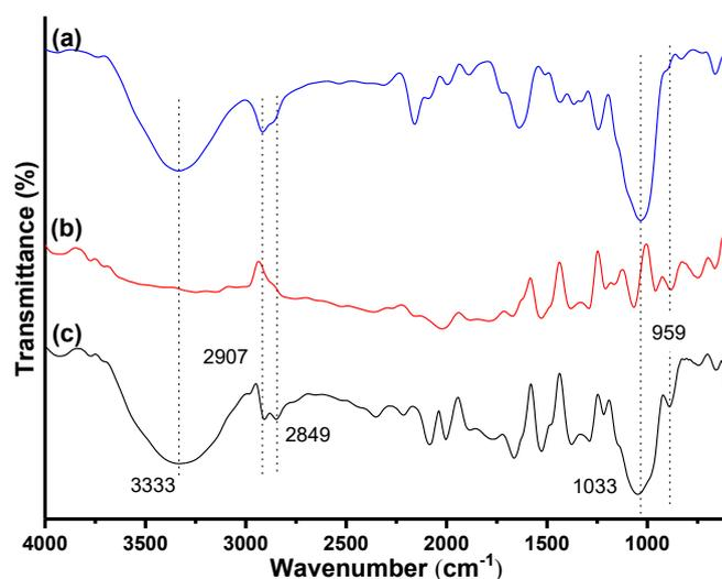
Fig 5. FTIR spectra of (a) the pure bamboo timber, (b) the  $\text{TiO}_2$ -coated bamboo timber, and (c) the superhydrophobic bamboo timber
