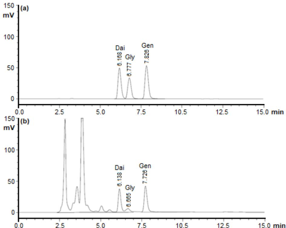
**Fig 6.** HPLC chromatograms of mixture standard solution (A) and soy milk sample solution (B) containing genistein (Gen), daidzein (Dai), and glycine (Gly). Mobile phase: methanol-water (63.26:36.74). Flowrate: 0.81 mL/min. Column: C<sub>18</sub> column of Hibar® 250-4,6 Purospher® STAR RP-18 endcapped (5 μm). Column temperature: 45.31 °C. Wavelength detection at 260 nm. Volume injection: 10 μL
