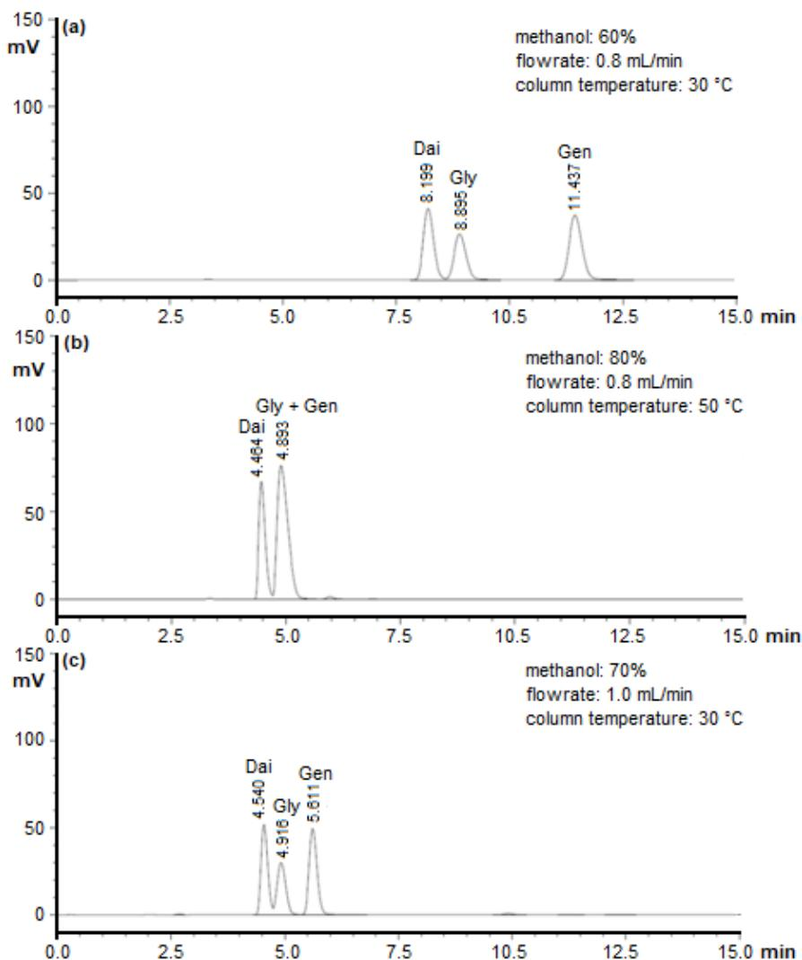
**Fig 2.** Preliminary HPLC optimization using three variations separation condition of OVAT1 (a), OVAT2 (b), and OVAT3 (c) for mixture standard solution containing genistein (Gen), daidzein (Dai), and glycine (Gly). Column: C<sub>18</sub> column of Hibar® 250-4,6 Purospher® STAR RP-18 endcapped (5 μm). Wavelength detection at 260 nm. Volume injection: 10 μL
