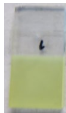
Fig 2. The thin film of CdS deposited by CBD
