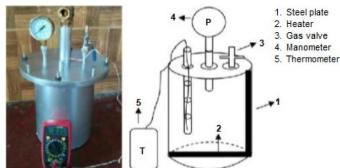
Fig 1. Scheme of HTC Reactor without stirring system
