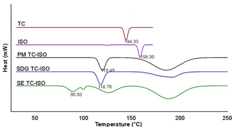
Fig 10. Thermogram profile of TC and TC-ISO 1:2 co-crystal
