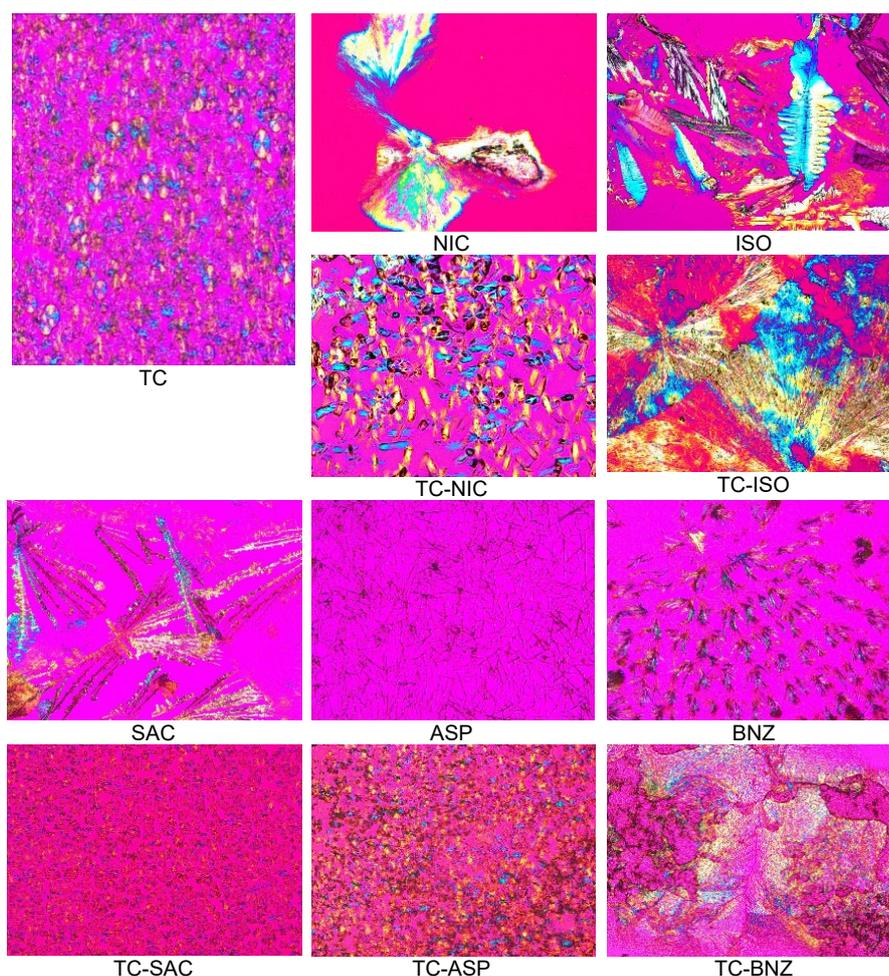
**Fig 4.** Polarizing microscopy of mixed TC and cofomers
