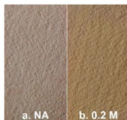
**Fig 10.** Change in the color of paper strip soaked in NA ( $1 \times 10^{-3}$  M) after the addition of  $S^{2-}$  (0.2 M)
