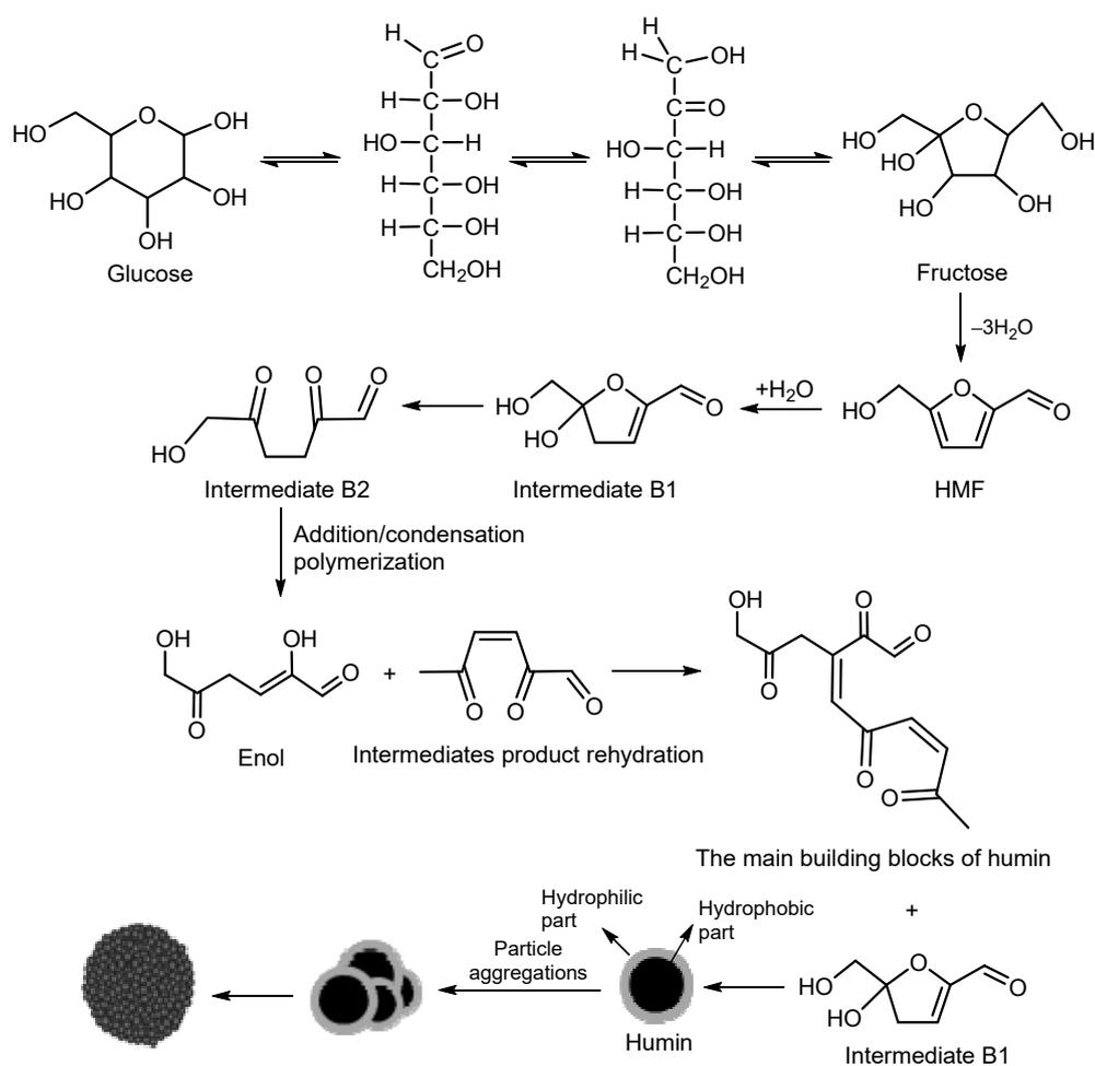
Fig 3. Mechanism of humin formation [32]
