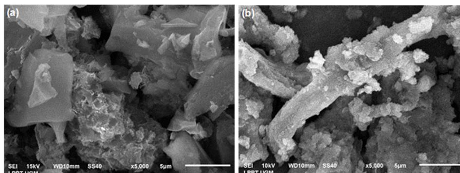
**Fig 7.** SEM of humin from (a) biochar 2:1 and (b) solid hydrolysate
