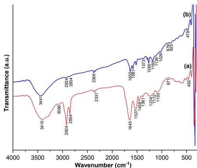
**Fig 4.** FTIR spectra of (a) humin from solid hydrolysate and (b) humin from biochar 2:1
