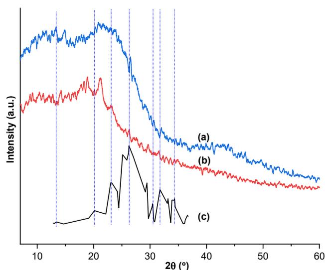
Fig 5. Diffractogram of humin from (a) biochar 2:1, (b) solid hydrolysate, and (c) JCPDS of Fe
