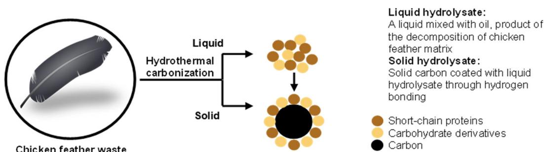
Fig 1. Hydrolysate formation from the hydrothermal carbonization process [8]
