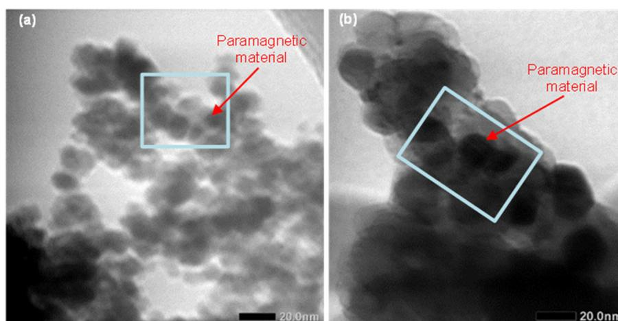
**Fig 6.** TEM image of synthetic humin from (a) biochar 2:1 and (b) solid hydrolysate
