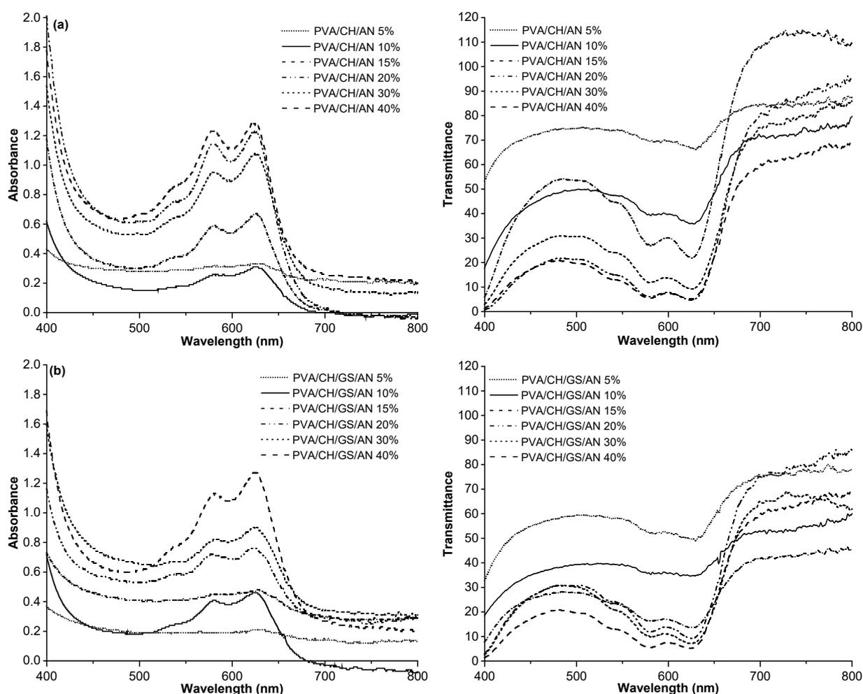
Fig 4. UV-vis film: (a) PVA/CH/AN and (b) PVA/CH/GS/AN
