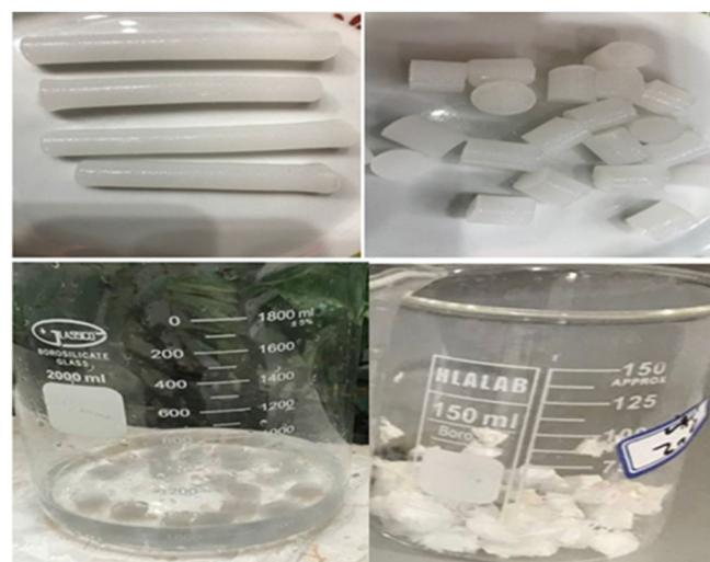
**Fig 1.** Image of a superabsorbent ZnO-loaded SA-g-poly (Ac-co-EBS) hydrogel composite
