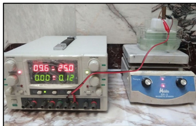
Fig 1. The electrochemical apparatus used to prepare the TiO 2 /ZnO nanocomposites
