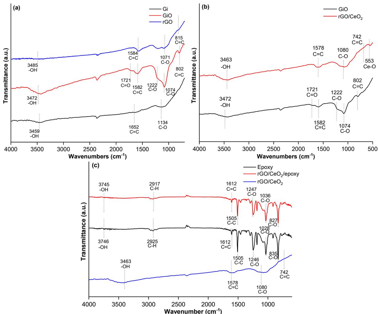
**Fig 4.** (a) FTIR spectra comparison of Gi, GiO, and rGO, (b) FTIR spectra comparison of GiO and rGO/CeO<sub>2</sub>, and (c) FTIR spectra comparison of epoxy, rGO/CeO<sub>2</sub>, rGO/CeO<sub>2</sub>/epoxy
