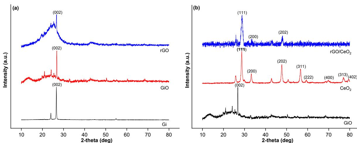
**Fig 2.** Diffractogram pattern of (a) Gi, GiO, and rGO, and (b) GiO, CeO<sub>2</sub>, and rGO/CeO<sub>2</sub>
