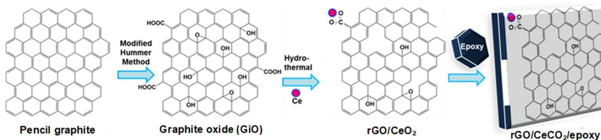
**Fig 5.** Schematic presentation for the synthesis of rGO/CeO<sub>2</sub>/epoxy composite
