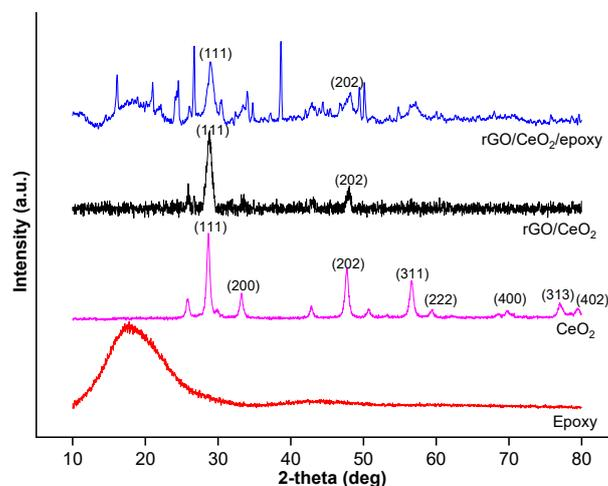
**Fig 3.** Diffractogram pattern of epoxy, CeO<sub>2</sub>, rGO/CeO<sub>2</sub>, and rGO/CeO<sub>2</sub>/epoxy composite
