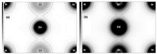
Fig 6. (110) Electronic density cubic (a) InZnCl<sub>3</sub> and (b) InCdCl<sub>3</sub> perovskites
