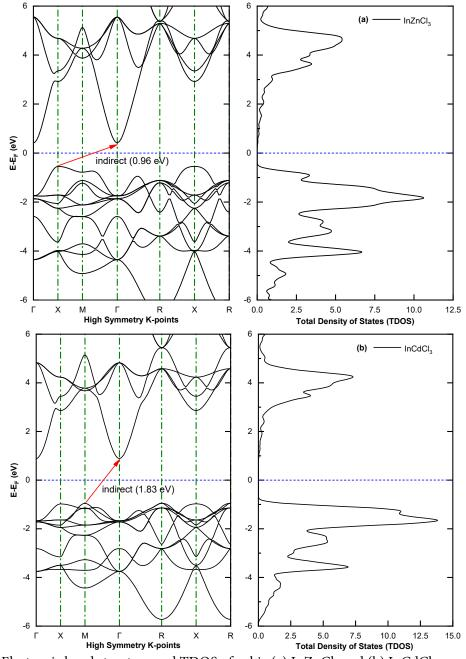
Fig 4. Electronic band structure and TDOS of cubic (a) InZnCl<sub>3</sub> and (b) InCdCl<sub>3</sub> perovskites
