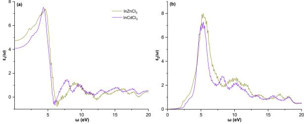
**Fig 7.** (a)  $\varepsilon_1(\omega)$  and (b)  $\varepsilon_2(\omega)$  of cubic InZnCl<sub>3</sub> and InCdCl<sub>3</sub> perovskites
