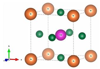
Fig 1. The unit cell structure of cubic InCdCl<sub>3</sub> perovskite material
