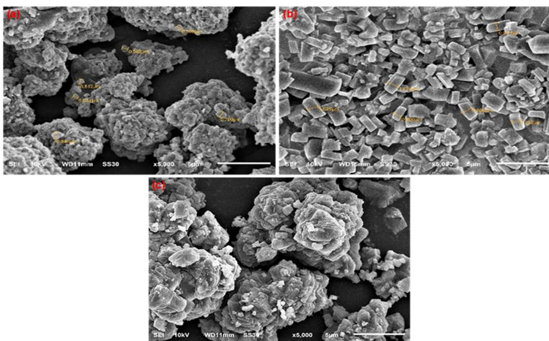
**Fig 6.** SEM test results on NCA cathode obtained from (a) citric acid leaching, (b) sulfuric acid leaching, and (c) precursor
