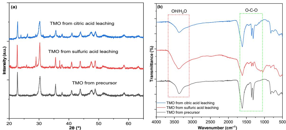
**Fig 3.** Comparison of (a) XRD patterns and (b) FTIR spectra of TMO from leaching using citric acid, sulfuric acid, and precursor
