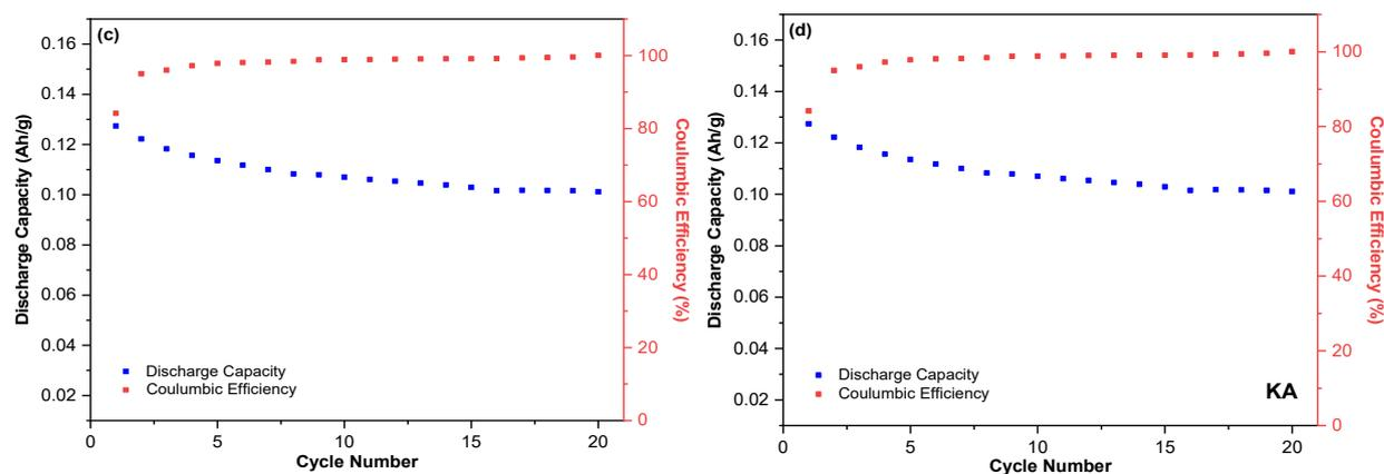
**Fig 8.** The charging-discharging cycle's performance characteristics on NCA are derived from (a) citric acid leaching, (b) sulfuric acid leaching, (c) precursor, and (d) commercial. The current used in the cycle is 200 mA/g (1 C)
