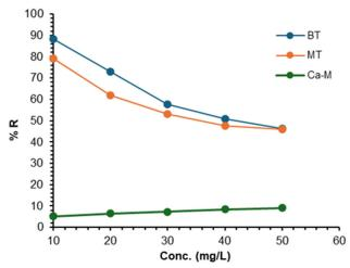
**Fig 4.** Removal percentage of BS dye as a function of its concentrations
