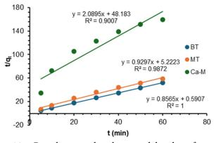
**Fig 11.** Pseudo-second-order model plot for the adsorption of BS dye onto clay samples at 298 K
