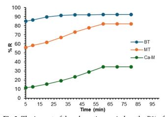
**Fig 3.** The impact of the adsorption period on the R% of BS dye
