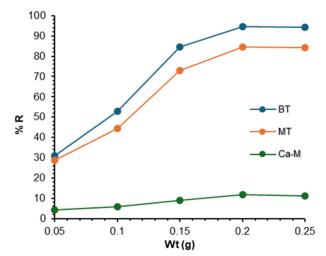
Fig 2. Effect of clay sample weight on the R% of BS dye
