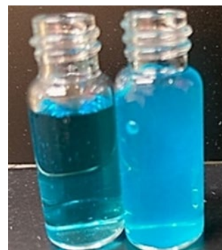
Fig 3. Cu(OH) 2 formation in CuCl 2 ·2H 2 O solution after the addition of NaOH at pH of 3.2 (left) and 3.5 (right)
