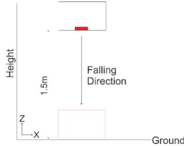
Figure 3 Vertical Fall Motion Scenario
