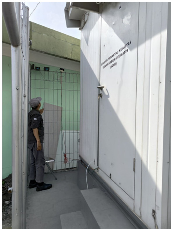
Figure 10. Installation of Iot-based LCS next to AQMS for calibration
