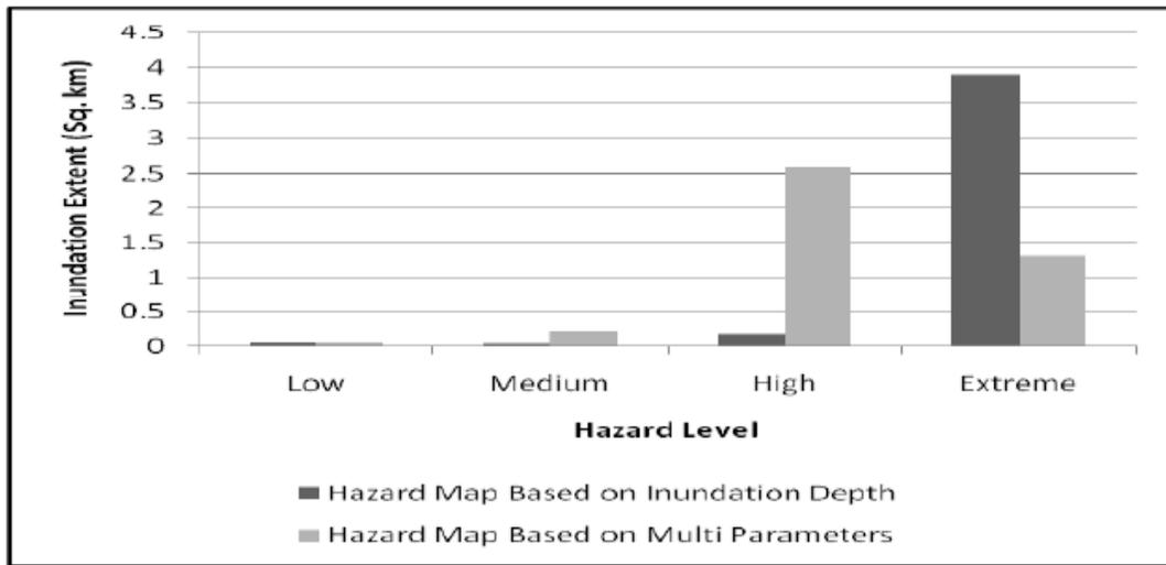
Figure 10. Inundation extent of each hazard class in single and multi parameter approach
