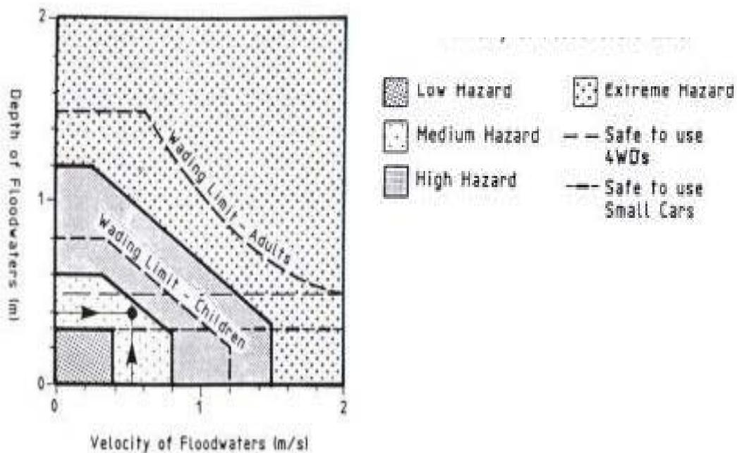
Figure 3. Hazard classification [Ramsbottom et. al, 2003]
