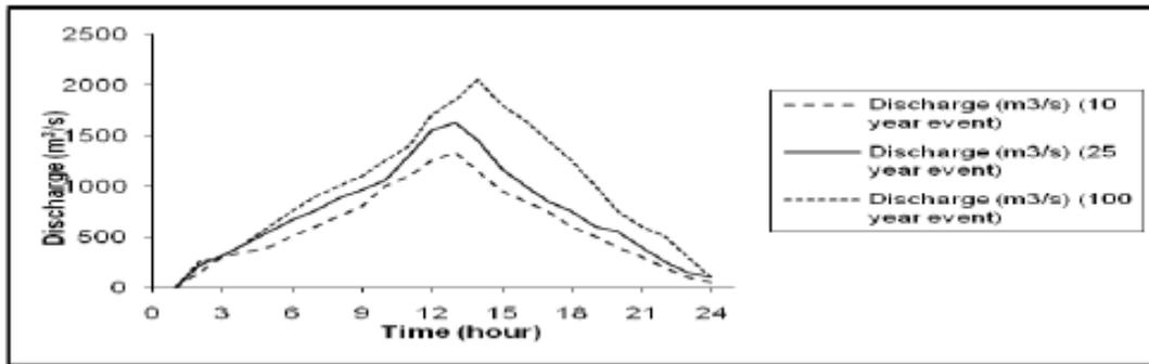
Figure 4. Hydrographs chosen as model input for three different return periods
