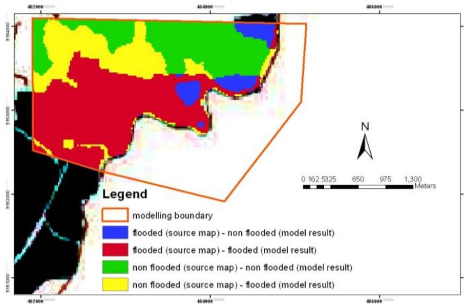
Figure 7. Overlaid between modelling result map and reliable source map flood hazard mapping
