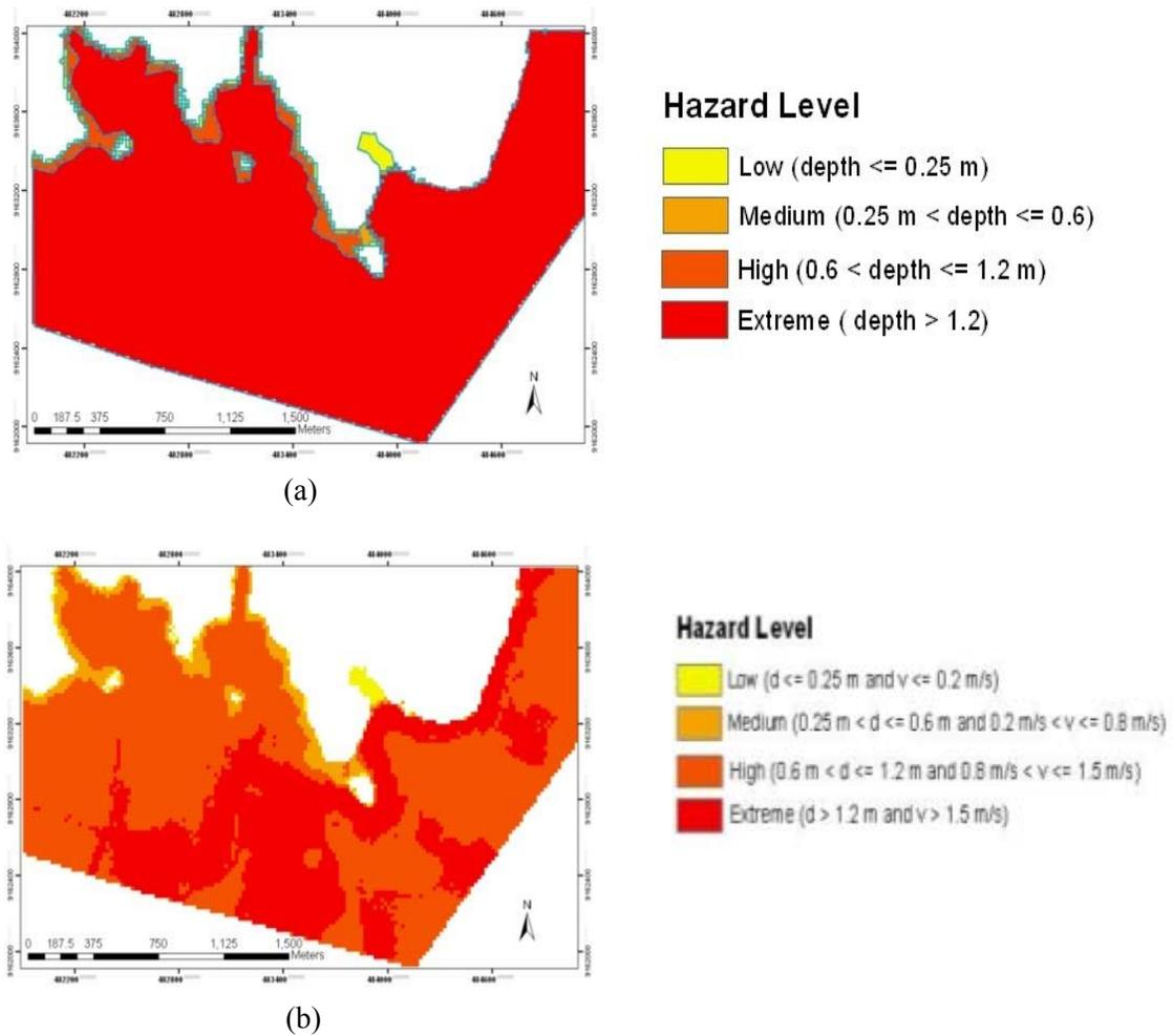
Figure 9. Comparison between single parameter map and multi parameter hazard map of 100 year return period. (a) Single parameter hazard map. (b) Multi parameter hazard map
