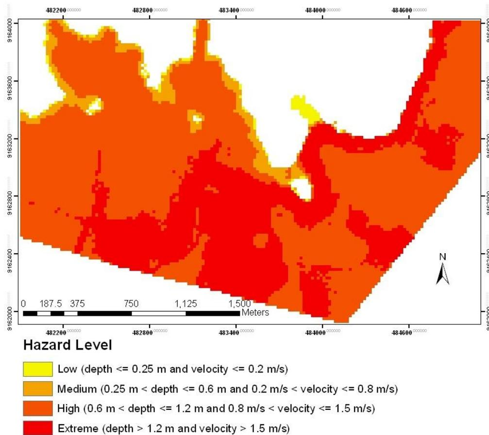
Figure 8. Flood hazard map based on multi parameters
