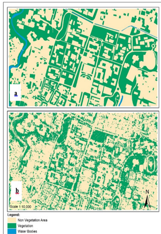
Figure 5. Comparison of vegetation area values from two methods (a) Image visual analysis and (b) Normalized Index calculation.
