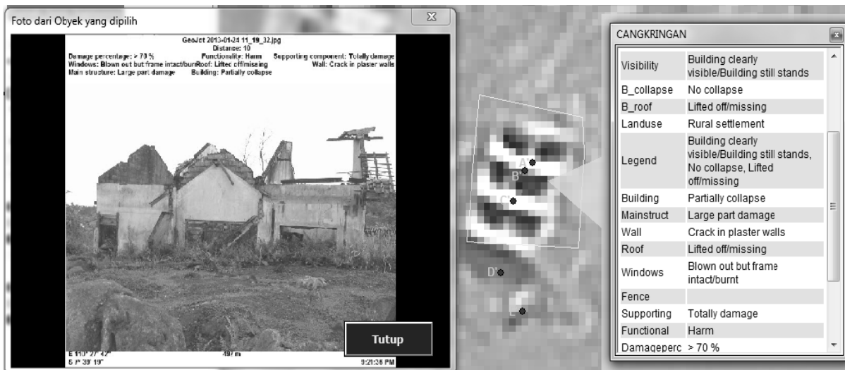
Figure 7. Combined geotagged photograph attribute and imagery interpretation attribute using GIS (spatial join process)
