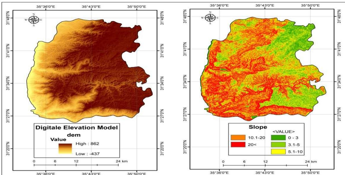
Figure 2. Digital elevation model and slope map for the study area.
