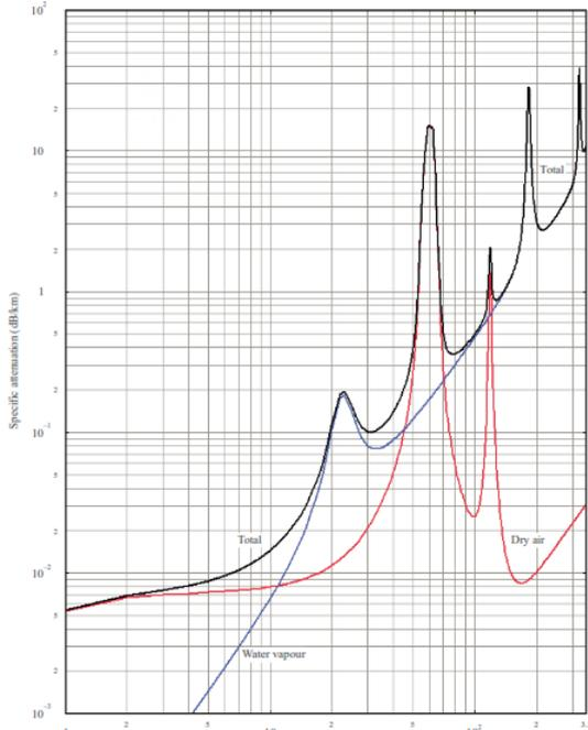
Fig. 1 Characteristics of atmospheric attenuation.
